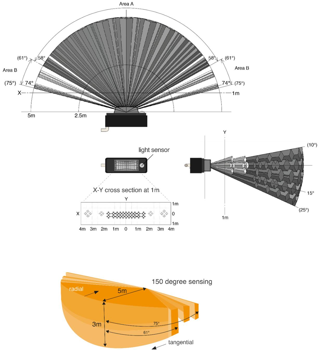
Figure 1 Detection area: X-Y cross section at 1m
