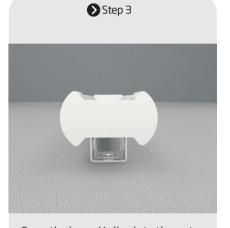
Snap the inner U clips into the outer clips orderly.
