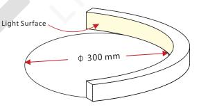
The light can only be bent along the light surface. Do not bend smaller than allowed minimum bend diameter.
