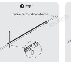
Thread the strap through the mounting profile and then cover it with silicone anti-skidding sleeve. Be attention to the direction when strapping.
