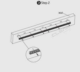
Mark the mounting positions and tighten screws.
